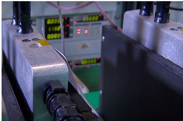
A KiWi smart-inverter undergoing HALT
